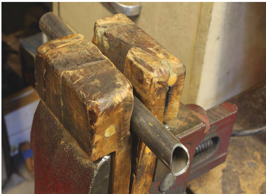
Battle-scarred DIY vise blocks hold tubing secure with no marks on the tube. They are made from shipping skid scrap and have been in service about 40 years. The base of the front one inside the vise is curved to allow it to align with odd shapes. It took 45 seconds, including changing from a cut-off disc to a sanding disc, to contour the tubing end.
