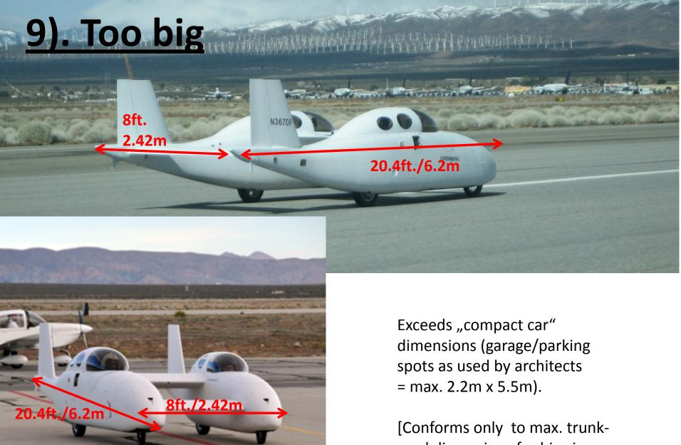
[Conforms only to max. trunk-road dimensions for big-rigs = max. 8.5ft./2.6m.]
