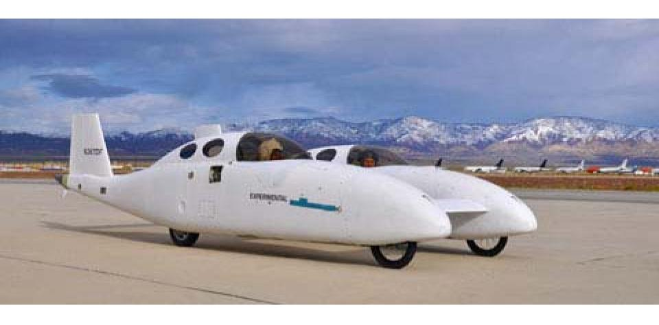
Small-diameter tires limit road-speed. Round-section tires reduce road-grip for cornering/braking.
