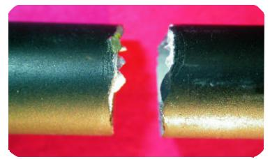
Photo B: A real close up of the two broken ends of Gilbert's control rod
