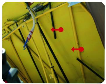
Photo A: Still in-place, but broken, control rod at the scene of Gilbert Goodlett's crash. This rod failed in fatigue after only a few hundred hours. A possible answer to, how was this possible, is that this rod was anodized to increase the ship's curb appeal
