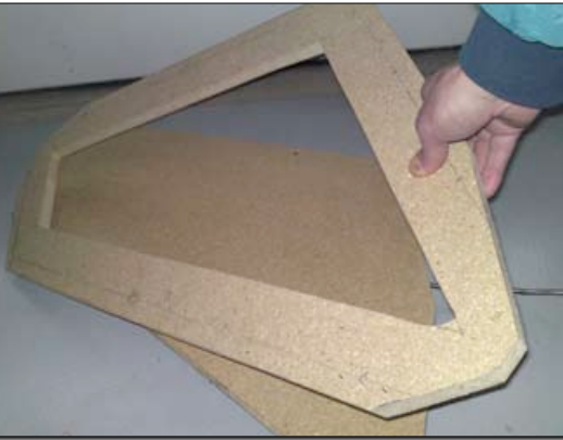
The first step in creating a new, bulging side window was to make a frame to define the mating flanges.
