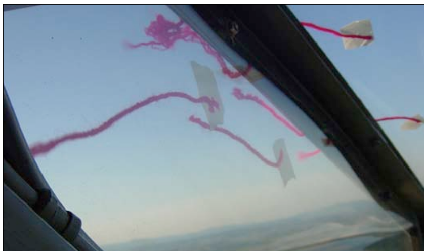
The tufts in flight. Yarn at the leading edge of the wing hangs there, indicating stalled airflow.
