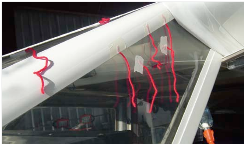
Tuft testing of the side window helped shine a light on local flow separation.
