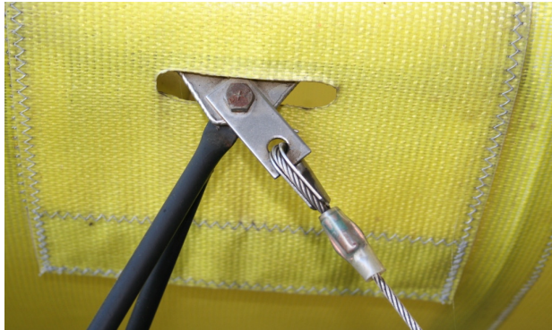
Figure 8.1: bracing cable termination on a Thruster T600N. The Thruster wing is strut and cable braced; this is the front spar, jury strut, inner flying wire connection point (as per figure 7.3b).
