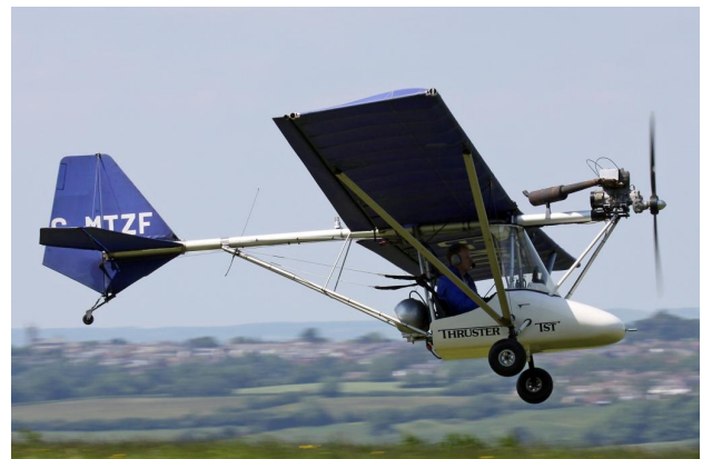
Figure 2.3: Thruster TST. Highly successful microlight of the late 1980s. Engine, wings and empennage all attach to the single, large diameter, aluminium fuselage tube (Curtis, H).
