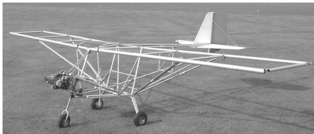
Figure 7.5: Sky Ranger minus covers. Note the two spar, or ladder frame, wing, two lift struts and structural jury struts. The wing's aerofoil shape is achieved by shaped, tubular battens that stiffen the sailcloth covers (Flylight Airsports).
