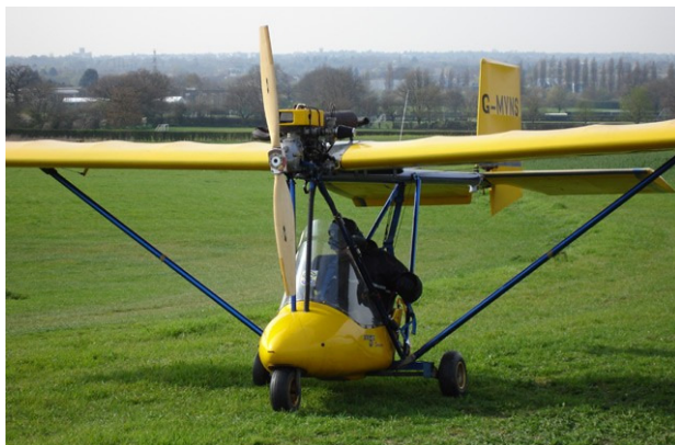
Figure 7.6: Mike Whittaker MW5. An example of a tubular single spar wing.
