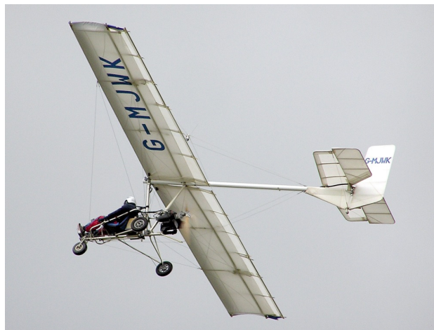
Figure 1.1: Huntair Pathfinder. Early microlight aeroplane featuring wire braced bolted aluminium tube construction, Dacron sailcloth covering and 2-stroke engine (Pingstone, A).
