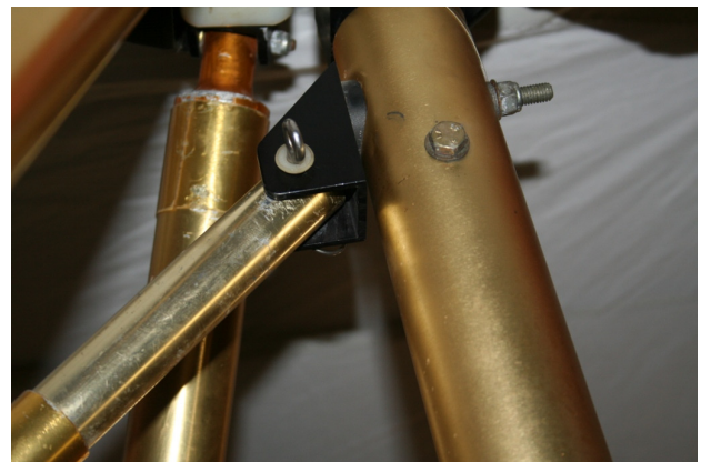
Figure 8.3: front strut (small diameter) to monopole (large diameter) attachment on a Pegasus XL-Q. This 'U' shaped bracket is cut from an aluminium extrusion.
