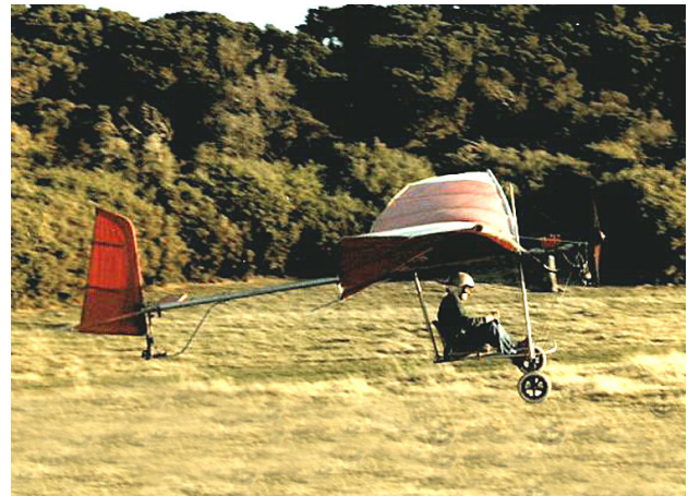
Figure 2.2: Skycraft Scout. Early microlight aeroplane clearly showing influence of Demoiselle.
