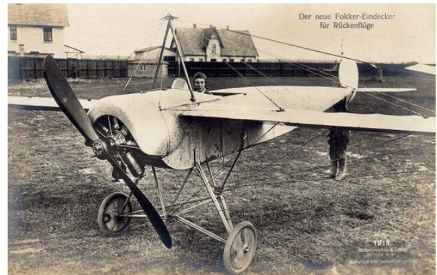
Figure 4.3: Fokker Eindecker. Wire braced mid wing monoplane fighter of WW1. A scale replica is available in the SSDR category.
