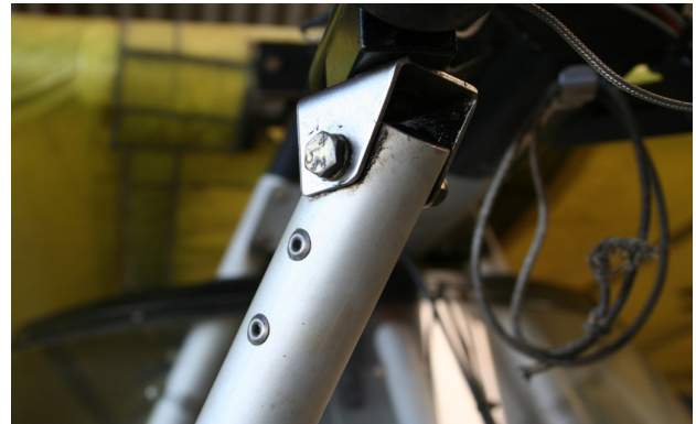
Figure 8.2: engine mount support strut on a Thruster T600N. The strut has a short inner sleeve riveted into the end. This increases the bearing strength of the bolt hole. The strut is bolted to a 'U' shaped bracket folded from stainless steel.
