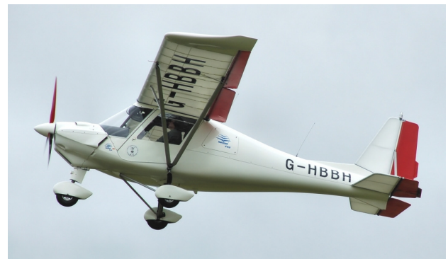
Figure 1.2: Comco-Ikarus C42. Modern microlight aeroplane, which is not dissimilar to a conventional light aeroplane. However bolted aluminium tube construction, and sailcloth wing covering, are retained (Pingstone, A).
