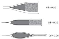
The amount of flow separation and the size of the wake have a large effect on drag. The streamlined body has the same frontal area as the others but much lower drag.
