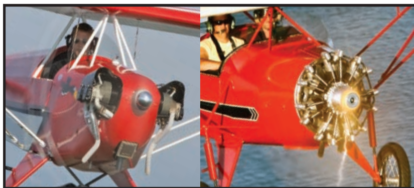
Comparison of the Baby Ace cowl (left), and the rounded nose Tim Gallagher designed for his radial engine.
