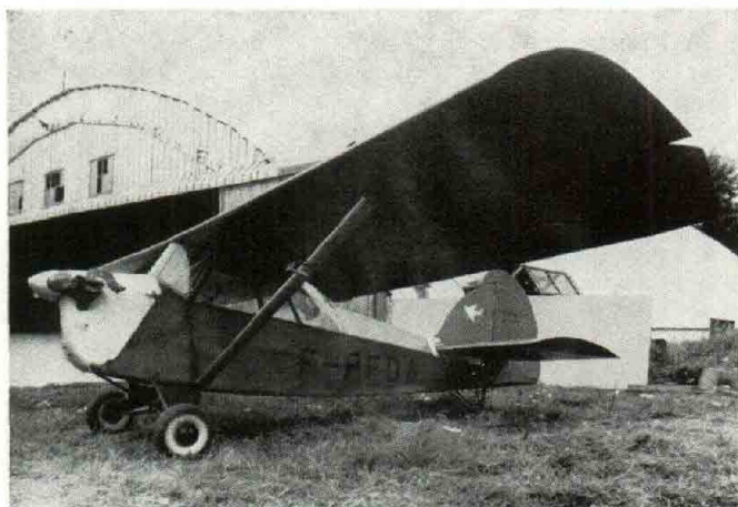
"L'Alouette", the Statoplan .01. Note thick section used in horizontal tail.
