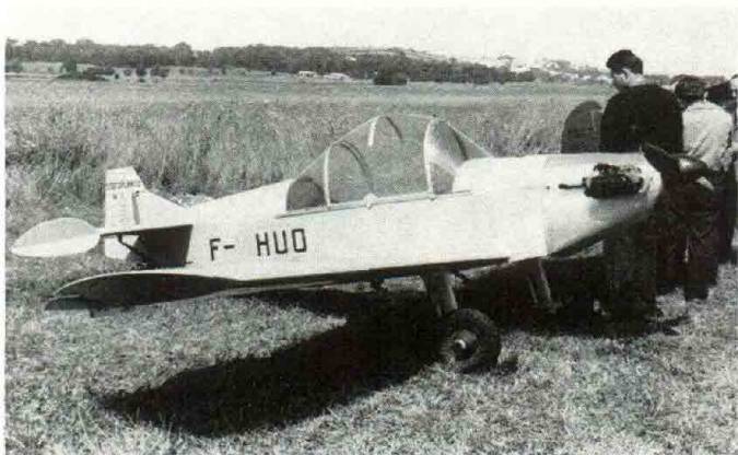
Little but good! The Statoplan .02 built by M. Gatard of France. Power is a converted Volkswagen engine. Note large canopy.
