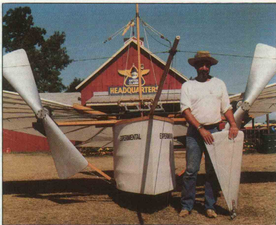
Andy Kosch holds a replica of the original Whitehead propeller. The two Whitehead types on the airplane are for tests.
