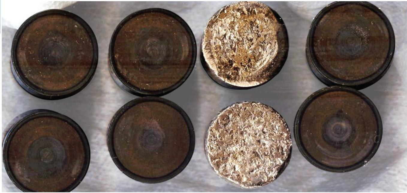
If the aircraft has been inactive for months preceding the prebuy exam, it may be prudent to pull some lifters to inspect them and the cam lobes for pitting or spalling.
